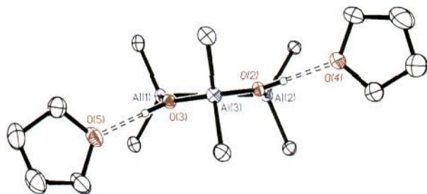
Figure 8. Core structure of [(t\text{Bu})_2\text{Al}(\mu\text{-OH})]_3 \cdot 2\text{THF} ( 6 ) viewed along an \text{Al}(3)\text{---O}(1) vector, showing both the twist-boat conformation of the \text{Al}_3\text{O}_3 ring and the positioning of the THF ligands. The tert -butyl methyl groups are omitted for clarity.
